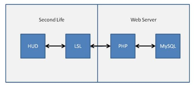
Figure 1 – Architecture diagram of the VASI (VCDI).
